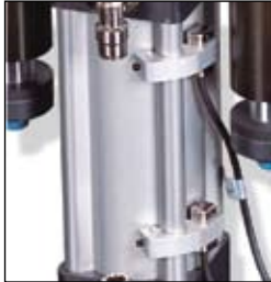
proximity switches are available for sensing end of travel
